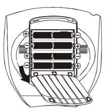
**NOTE:** In order to operate the unit on battery power the AC cord must be disconnected from the AC socket on the back cabinet.
